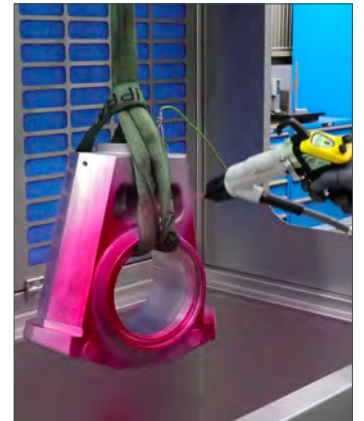
Electrostatic application of testing agent at a penetrant station
